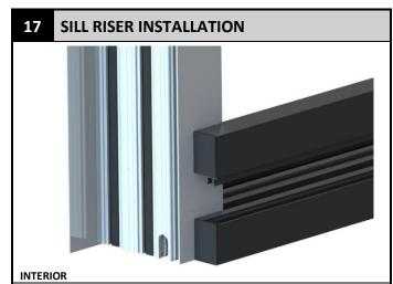
Align the riser with the interior sill channel. Tap the riser until it snaps into the channel and both barbed legs are fully engaged. Gently clean excess sealant that may have squeezed out taking care not to remove sealant at the joint.
