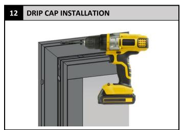
With the drip cap in place predrill holes for installation fasteners. Using 3/16" bit drill holes through the drip cap and the nailing fin (approximately ½" from top of fin). Place holes 4" from each end and spaced every 4"-8" on center.
