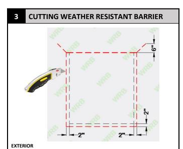
Cut the house wrap at the sill 2" below the rough opening and 2" past the jambs on each side. Cut the house wrap at the head even with the framing and diagonally past the jambs 6" to create a flap.
