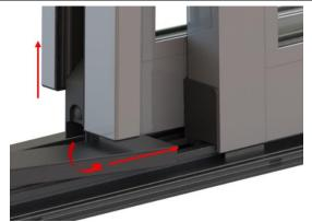
For 4-Wide doors, open passive panel completely, and lift front end. While panel is lifted, slide sill track cover into position under panel boxes, following alignment in step 21 (a). Apply pressure until the legs snap into place. Scan QR Code below for example video.
