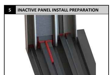
At the jamb to sill corner of the inactive panel, apply a generous amount of sealant around all seams of the frame filler block as shown. Also, apply a bead of sealant approximately 4" from the end, between the two pieces of foam tape.
