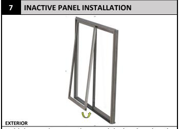
Hold the panel at an angle toward the head track and insert the top of the panel into the exterior most head track. Swing the bottom of the panel in until it is vertical. While in the lifted position slide the inactive panel against the inactive side jamb. Then gently lower the inactive panel onto the sill track. This will ensure all sealant makes contact between inactive panel and frame. If necessary, run an additional cap bead of sealant by lifting panel and applying sealant.
