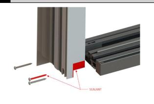
Insert the 3 sill attachment screws (A) through the predrilled holes in the bottom of the side jambs. Applying sealant to the top screw. Position the sill into place. Hold sill and side jamb tightly together as you tighten the screws. Clean off excess sealant that may have squeezed out taking care not to compromise the sealant at the joint.
