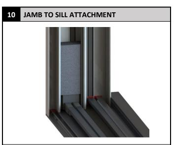
Position a foam block (J) into the stationary jamb track, using the squeeze out silicone from step 9 to secure the foam block to the sill track filler block.
