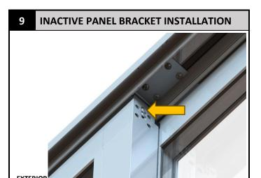
With the inactive panel tight to the inactive side jamb, loosen installed (M) screw, and slide bracket tight against head. Add (4)  $\#10 \times 5/8$ " SS pan head screws (B) through the installation strap into the pre-drilled holes in the head jamb.
