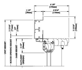
A - VERTICAL SECTION 3-1/2" ALUMINUM FLAT CASING (3-5/16" [84mm] ACTUAL SIZE)
