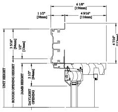
A - VERTICAL SECTION **ALUMINUM K STYLE CASING** (3-13/16" [97mm] ACTUAL SIZE)
