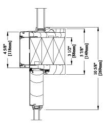
C - HORIZONTAL 3-1/2" [89mm] STACK SECTION (a)
