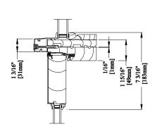
C - HORIZONTAL TIGHT STACK SECTION (a)
