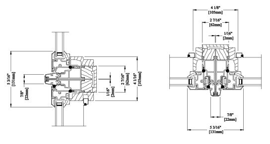
C - HORIZONTAL TIGHT STACK SECTION (a)
